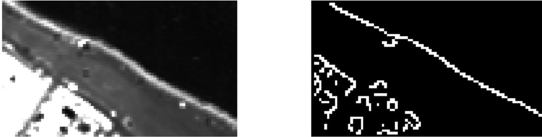
**Figure 9:** (a) Map of Modified Redness Index. (b) After Canny edge function is applied (Station 66)
