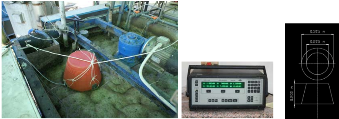
Figure 3: (a) photo of the configuration of the SBR with the floating container for the on line gas measurement, (b) instrument for the on line measurement of gas emissions and (c) cross section and side view of the floating container
