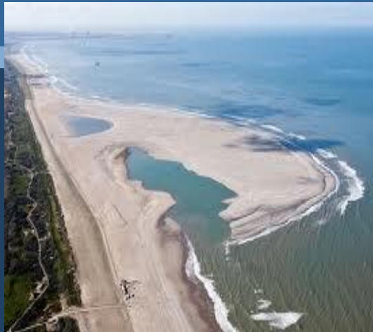
'Sand motor' beach replenishment, Ter Heijde, Netherlands
