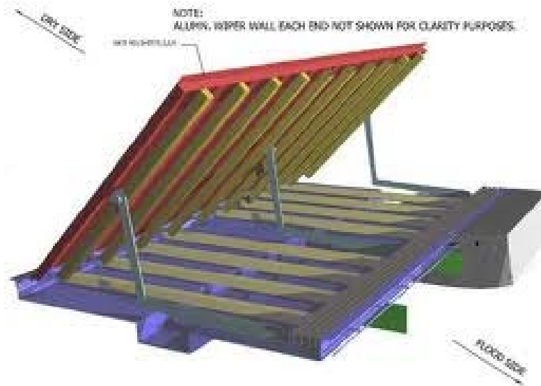
Figure 11: Passive Flood Barrier Floodbreak ®
