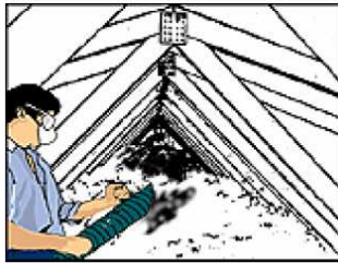
Blown-in attic insulation
