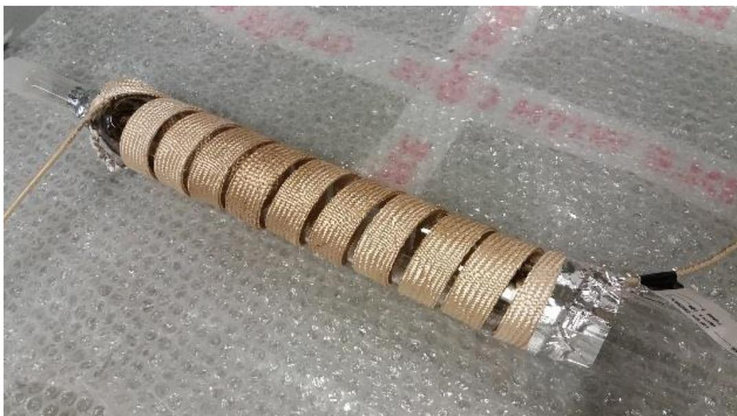
**Figure 3.** The quartz tube reactor with heating tape wrapped around its exterior (before the application of insulation).
