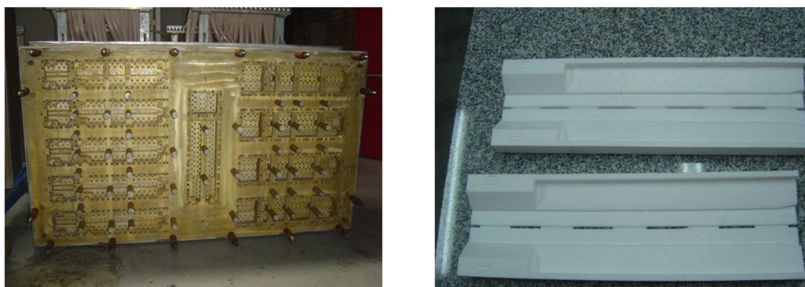
Figure 3. Designed mould (left) and EPS recycled prototype (right).
