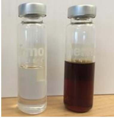
Figure 2: Color difference between pure glycerol (left) and unrefined/crude glycerol byproduct (right)
