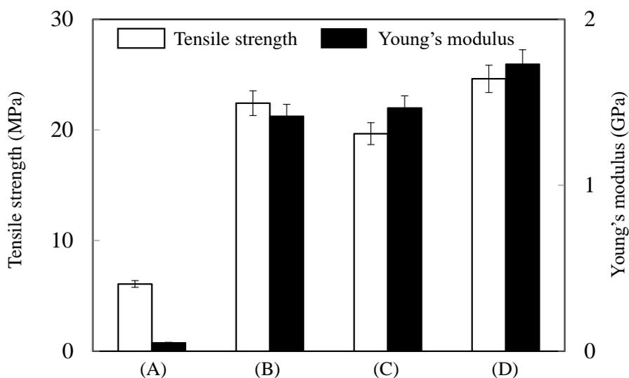
**Fig. 8** Tensile strength and Young's modulus of various composites. (A) PLA, (B) PLA with 5% CNF obtained from holocellulose, (C) PLA with 5% wtCNF obtained from  $\alpha$ -cellulose, and (D) PLA with 5% wtCNF (a commercial CNF, BiNFi-s WMa-10002)
