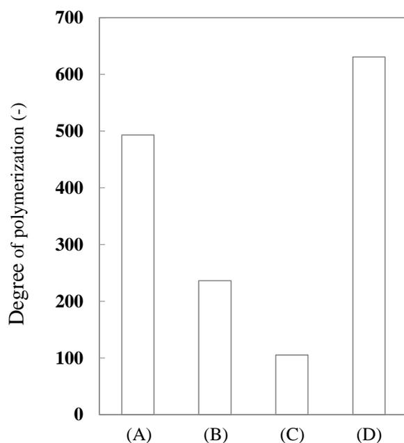
**Fig. 6** Degree of polymerization of  $\alpha$ -cellulose in residue after bleaching obtained from steam-exploded white poplar chopsticks waste and commercial cellulose nanofiber (BiNFi-s WMa-10002, Sugino Machine Ltd.). (A) 2.5 MPa and 5 min, (B) 3.0 MPa and 5 min, (C) 3.5 MPa and 5 min, (D) BiNFi-s WMa-10002
