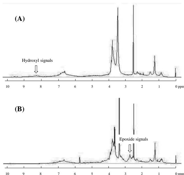
**Fig. 4** <sup>1</sup>H NMR of (A) acetone extract and (B) epoxidized lignin synthesized from acetone extract
