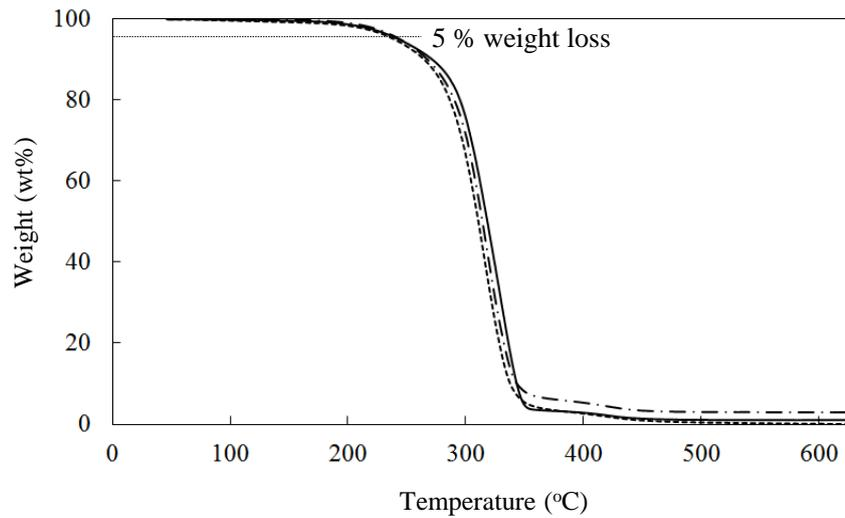
**Fig. 9** TG/DTA profiles of PLA and CNF/PLA composite. Solid line: PLA, dashed line: PLA with 5 wt% CNF obtained from holocellulose, and dotted line: PLA with 5 wt% CNF (a commercial CNF, BiNFi-s WMa-10002)
