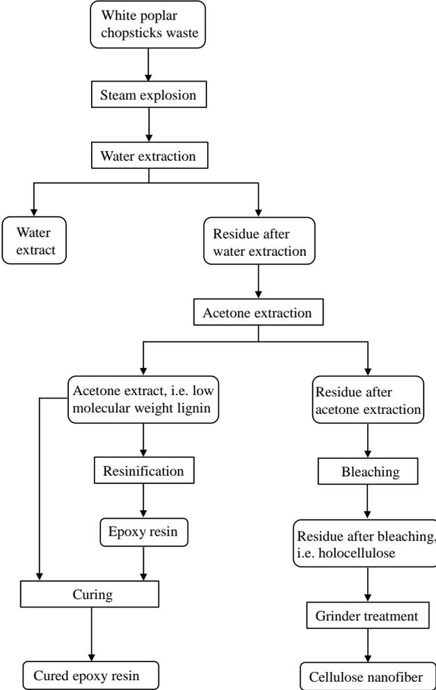
**Fig. 1** Flow chart of steam explosion followed by water and acetone extractions from white poplar chopsticks for cellulose nanofiber and cured epoxy resin co-product
