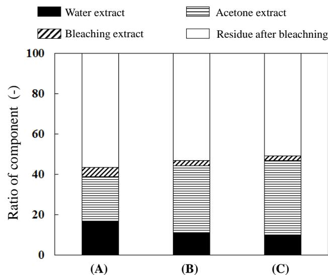
**Fig. 2** Ratio of component to dry weight of steam-exploded white poplar chopsticks waste. (A) 2.5 MPa and 5 min, (B) 3.0 MPa and 5 min, (C) 3.5 MPa and 5 min
