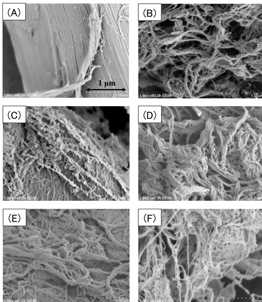
**Fig. 7** FE-SEM of (A) untreated white poplar chopsticks waste, (B) steam-exploded product at 2.5 MPa for 5 min, (C) residue after water extraction, (D) residue after acetone extraction, (E) residue after bleaching, and (F) cellulose nanofiber
