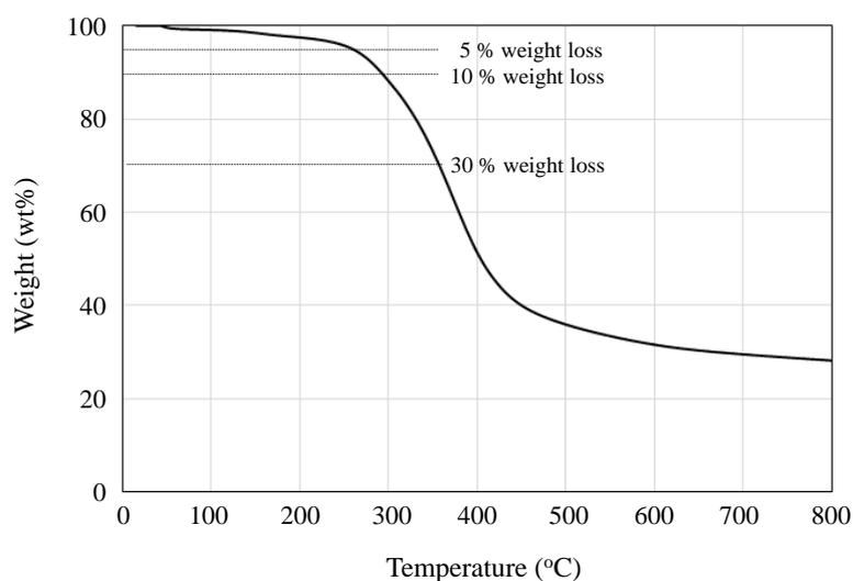
**Fig. 5** TG/DTA profiles of cured epoxy resin made from acetone extract, i.e. low molecular weight lignin
