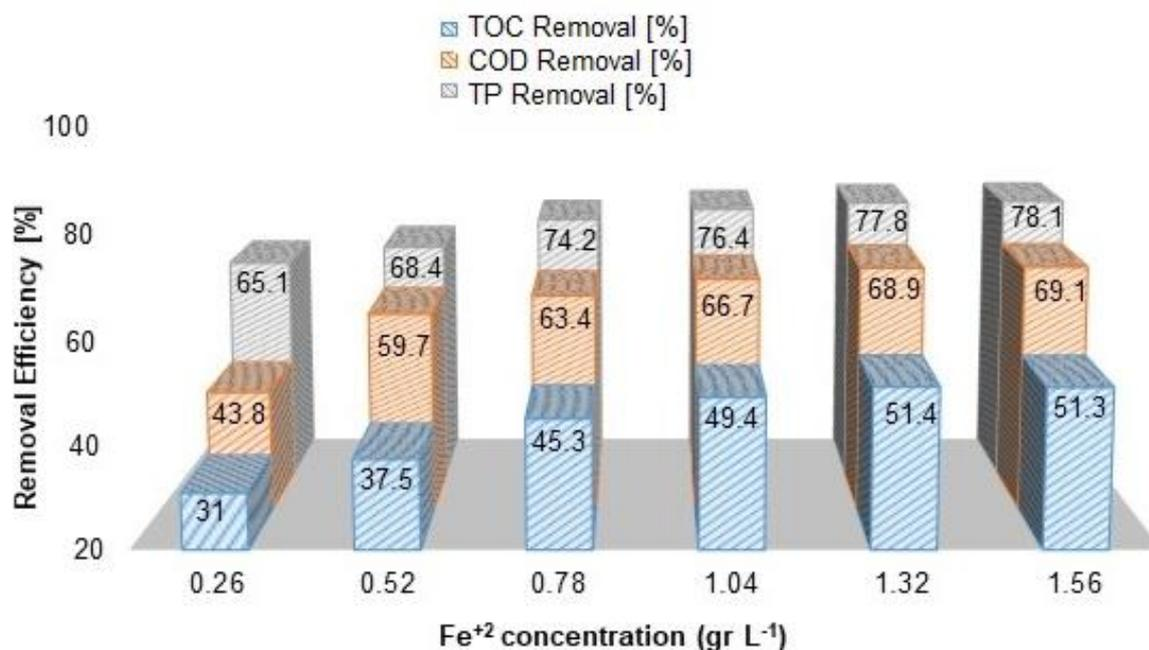
**Figure 2.** The effect of the  $\text{Fe}^{+2}$  concentration on the TOC, COD and TP removal.
