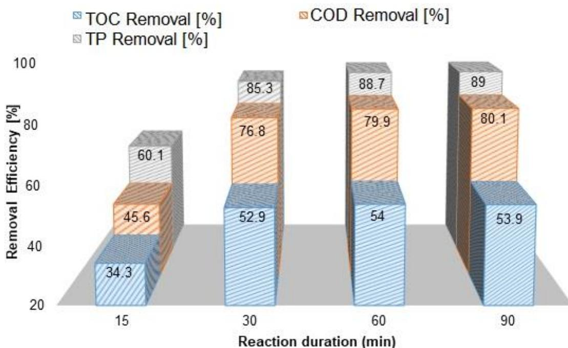
**Figure 5.** The effect of reaction duration on the TOC, COD and TP removal.
