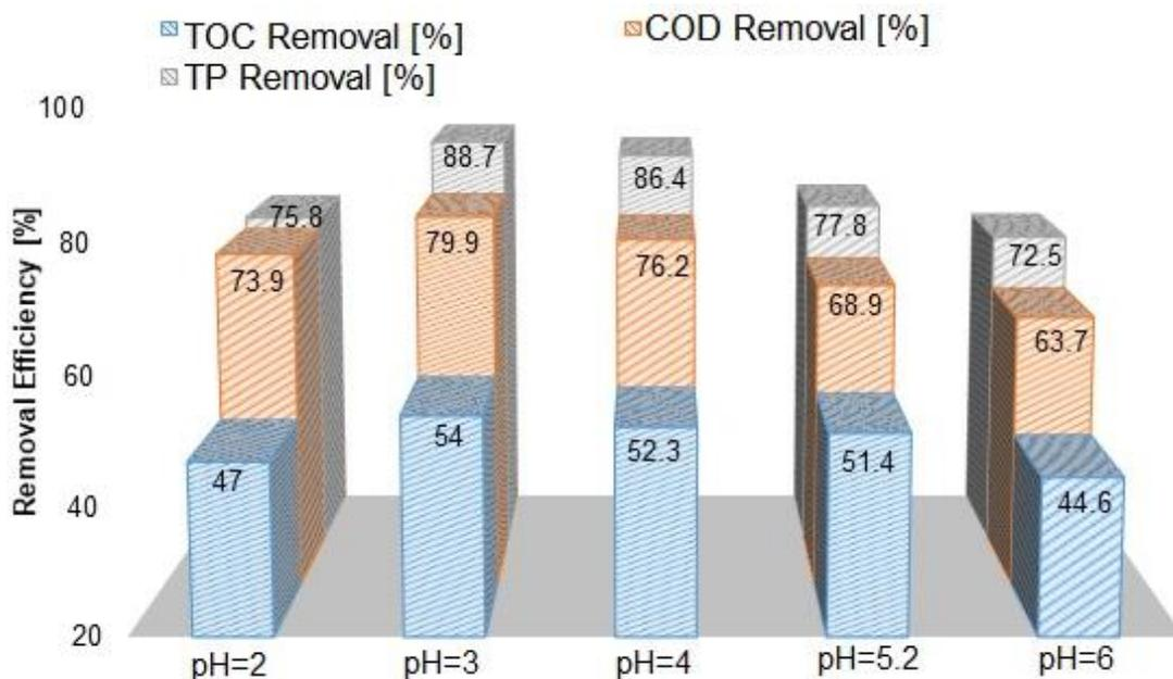
**Figure 4.** The effect of initial PPIW pH on TOC, COD and TP removal.
