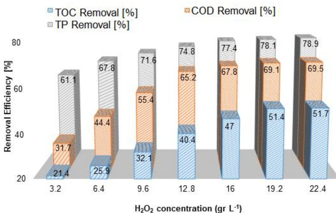
**Figure 3.** The effect of the H<sub>2</sub>O<sub>2</sub> concentration on the TOC, COD and TP removal.
