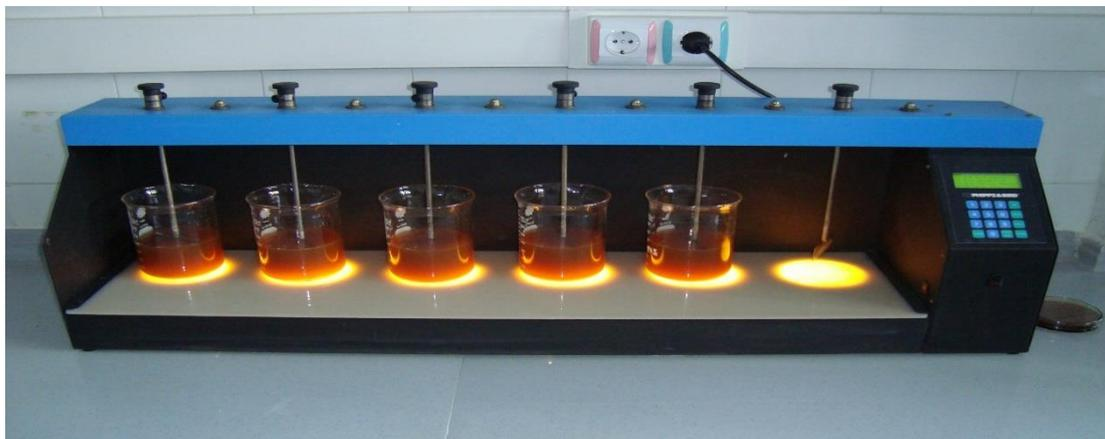
**Figure 1.** Schematic view of the experimental system for the lab-scale Fenton oxidation treatment of PPIW.
