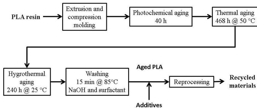
Fig. 1. Recycling process applied to PLA
