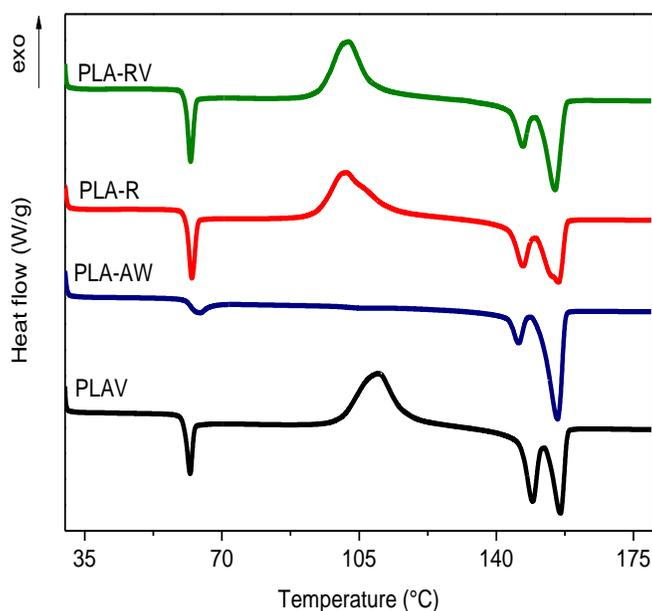
Fig. 3. First DSC heating scans of the different samples.
