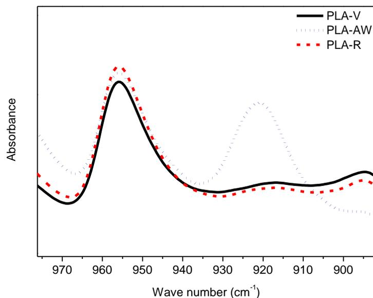
Fig. 2. Comparison of the band at 920  $\text{cm}^{-1}$  of PLA-V, PLA-AW and PLA-R.
