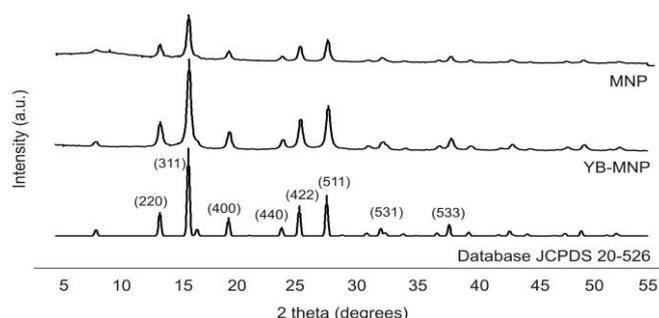
Figure 1. Powder X-ray diffractograms from representative MNP, YB-MNP and MNP from Database JCPDS 20-526 nanoparticles displaying the Bragg peak reflections of magnetite.
