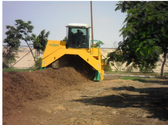
Photo 2: A pile during turning.
