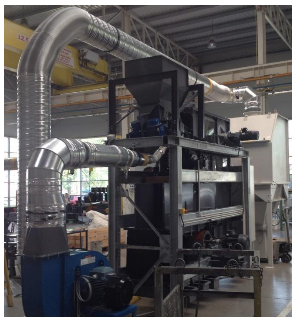
Figure 7. Photo of the 400 mm width KLME separator and auxiliary air system
