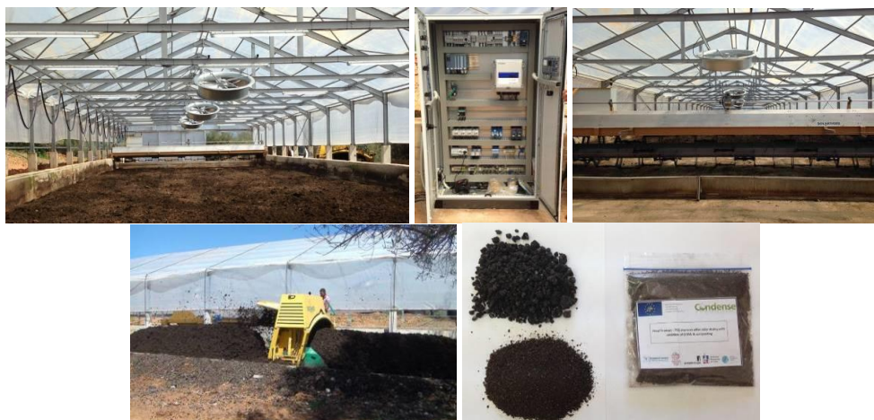
Picture 1. Solar drying unit and composting floor in the pilot unit in Iliia and the final product
