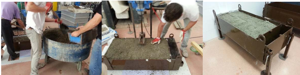
Figure 4. Sample preparation on UCLT test
