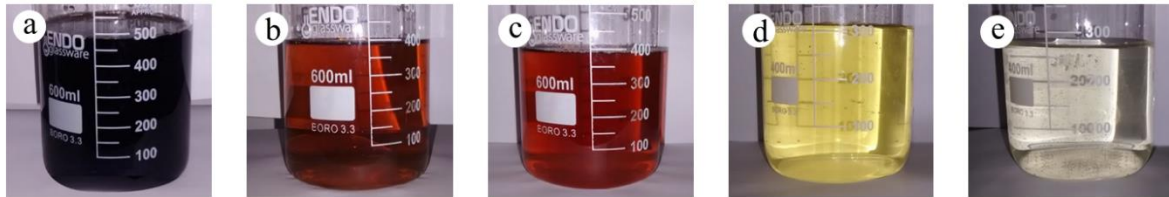
Figure 2. Visual observation of the landfill leachate at various stages of the treatment process: (a) raw, (b) after coagulation-filtration, (c) after chemical oxidation, (d) after geochemical reaction, (e) after reverse osmosis.
