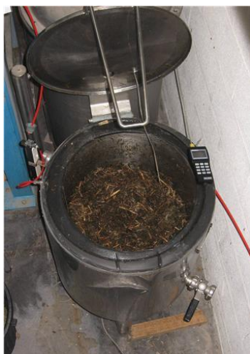
Fig1: 80 L composting reactor
