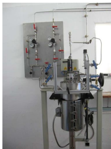
Fig. 2: 4 L Hydrolifiquefaction reactor
