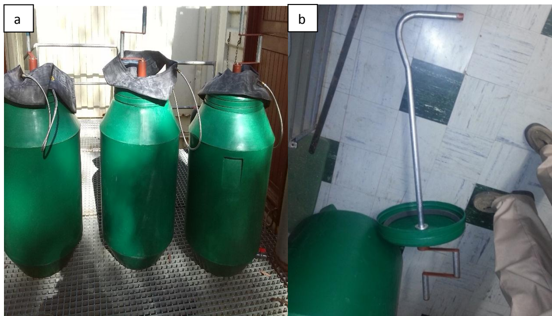
Figure III a: The second type of anaerobic digesters with the attached inner car tyre tube. Figure III b: The crank handle with the stirrer attached to the lid of the anaerobic digester. This was to permit stirring of the anaerobic digester contents.
