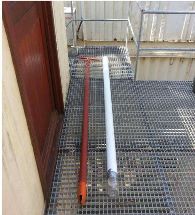
Figure I: The hollow sampler that was used to collect the pit latrine faecal sludge on the first sampling expedition with the plastic cover sleeve next to it.
