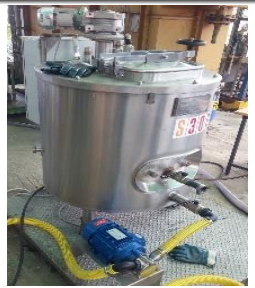
Storage of grinded OFMSW
