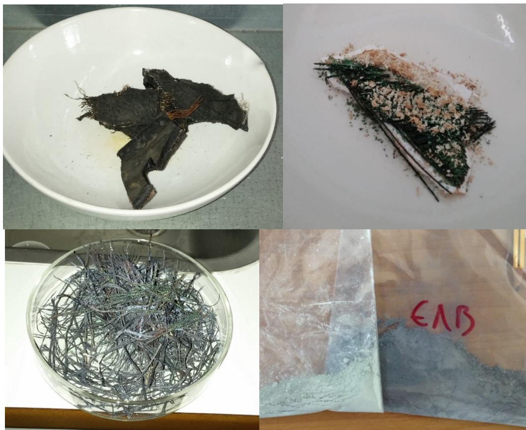
Fig 6 Top Left: sample before ashing, top right: sample after ashing, bottom left: separated wire, bottom right: ash collected
