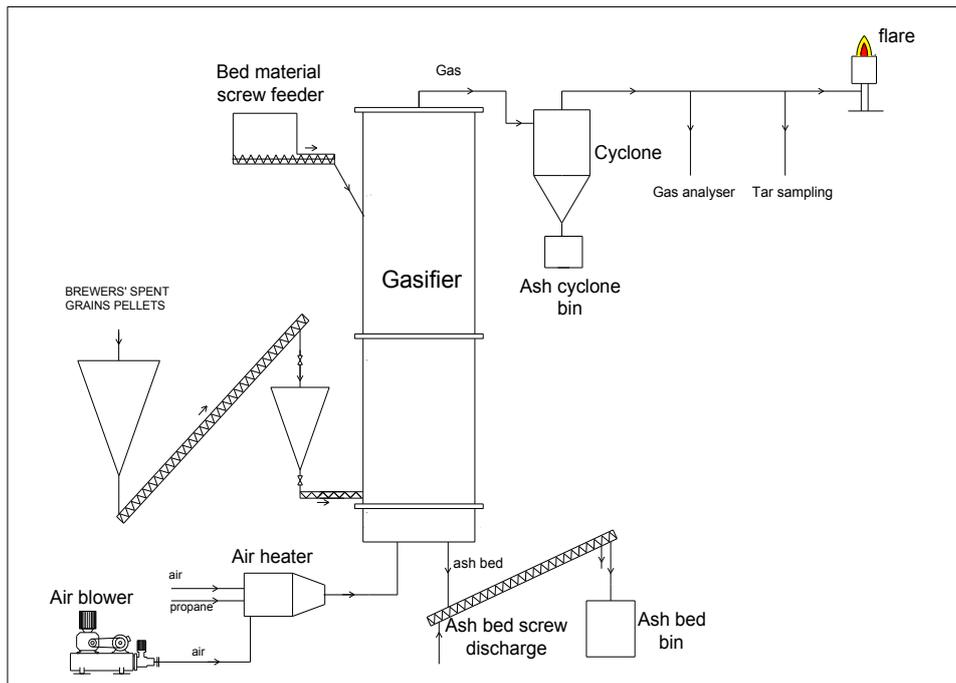
Figure 1. Experimental gasifier set-up.
