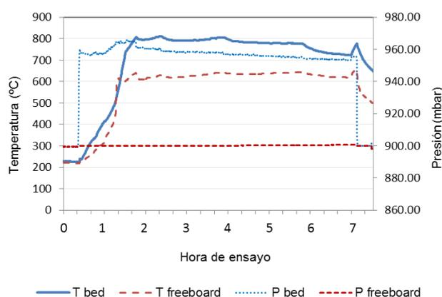
Figure 2. Bed and freeboard temperatures and pressure evolution
