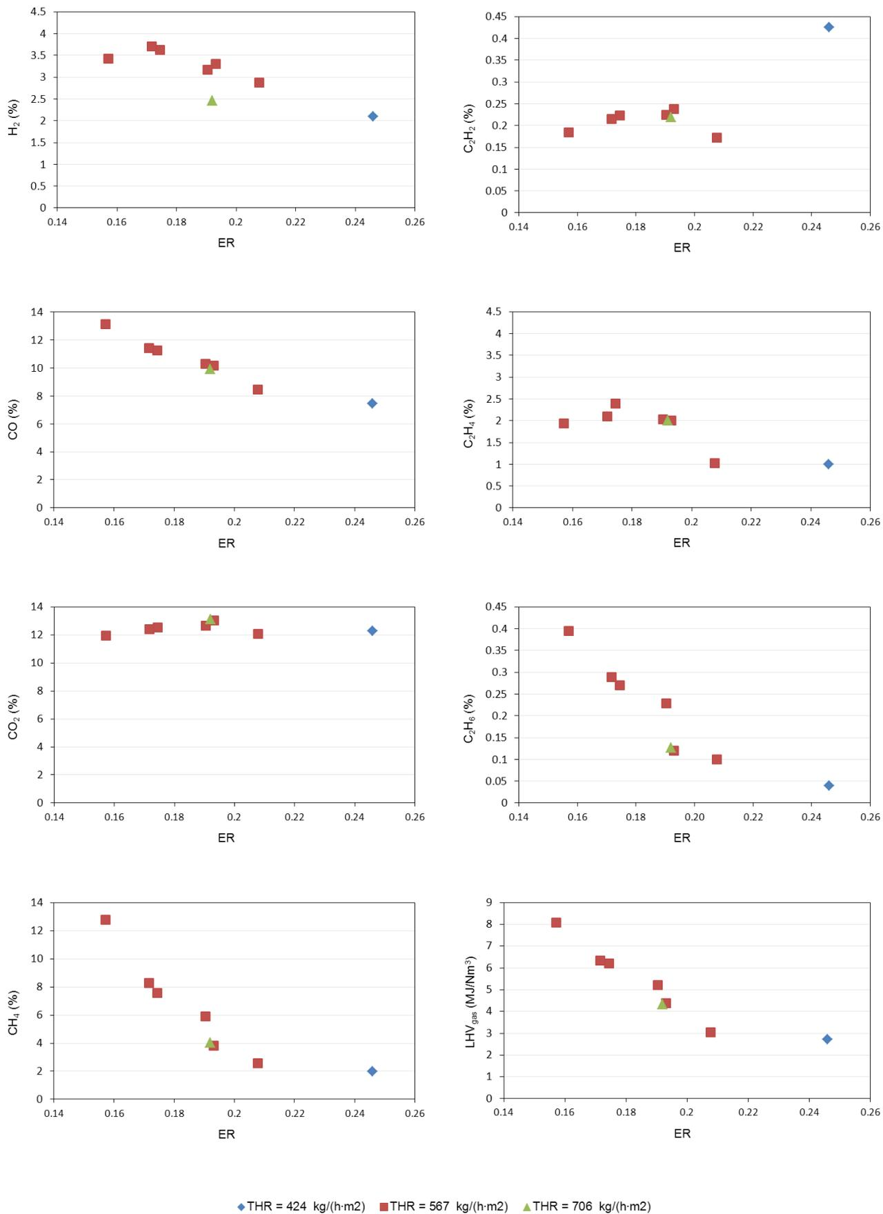
Figure 4. Gas composition and low heating value of the gas produced.
