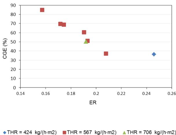
Figure 8. Cold gas efficiency of the gas produced as a function of ER.
