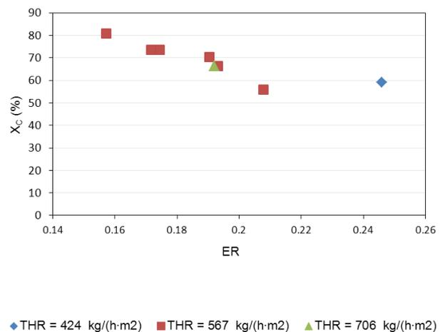
Figure 9. Carbon conversion gas produced as a function of ER.
