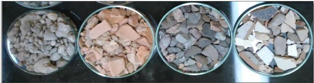
**Figure 3.1** - The components from the recycled aggregates (RA) after manual sorting
