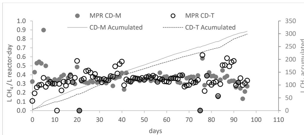
Fig.6 Comparison of daily and accumulated methane productions for CD-M and CD-T
