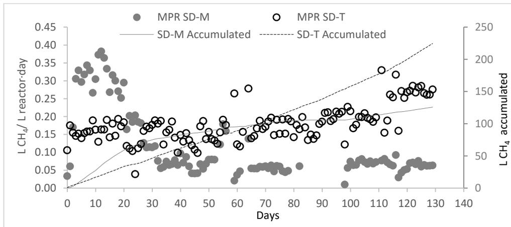
**Fig.5** Daily and accumulated methane productions for SD-M and SD-T
