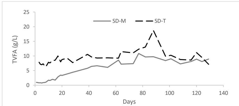
**Fig.2** Comparison of TVFA concentrations for SD-M and SD-T
