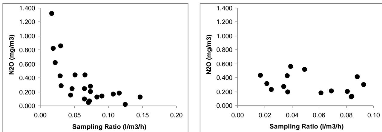
**Fig. 1:** (a)  $\text{N}_2\text{O}$  emission/SR-Fixed gas chambers, (b)  $\text{N}_2\text{O}$  emission/SR-Floating gas chambers
