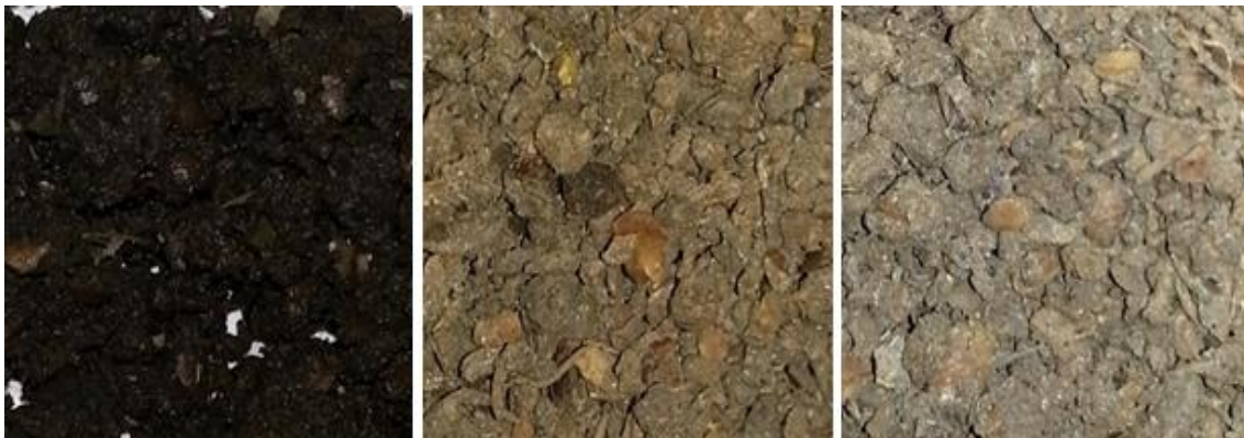
Fig. 3. Photographs of air-dried biogas digestate (1. dewatered digestate, 2. partially dried and 3. dried product)
