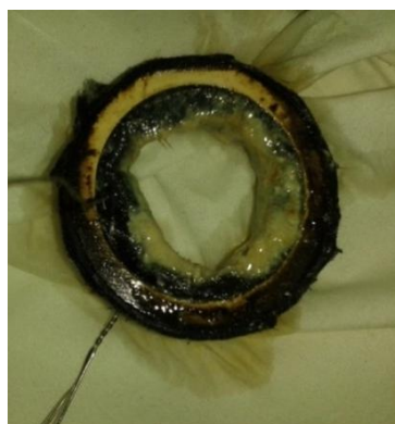
Figure 8. Photo of the anode chamber after 756.1 h of cell operation
