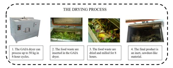
Figure 1. The process of drying and milling of food waste in a commecial GAIA dryer.
