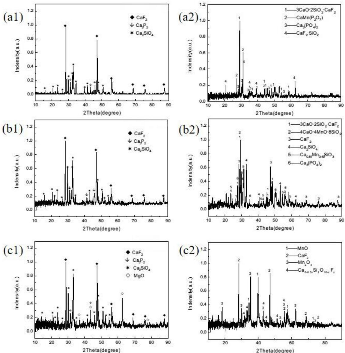
**Figure4 The XRD patterns of RDP slags and disposed slags (a1:1# RDP slag, a2:1# disposed slag, b1:2# RDP slag, b2:2# disposed slag, c1:3# RDP slag, c2:3# disposed slag)**
