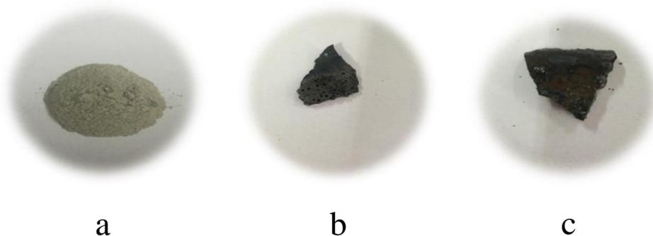
**Figure 6 Surface morphologies of disposed slag after 30 days exposed in the air (a:1# disposed slag, b:2# disposed slag, c:3# disposed slag)**
