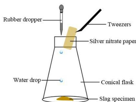
**Figure 3 The schematic diagram of discoloration detection with  $\text{AgNO}_3$  test paper**
