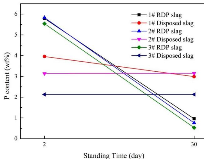
**Figure 5 Phosphorus content of slag variation after 2 and 30 days exposed in the air**
