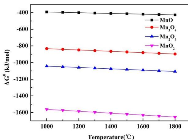
**Figure 2**  $\Delta G^0$  change of  $\text{Ca}_3\text{P}_2$  reacting with different manganese oxides ( $\text{MnO}_2$ ,  $\text{Mn}_2\text{O}_3$ ,  $\text{Mn}_3\text{O}_4$ ,  $\text{MnO}$ ) at temperature of 1000-1800°C
