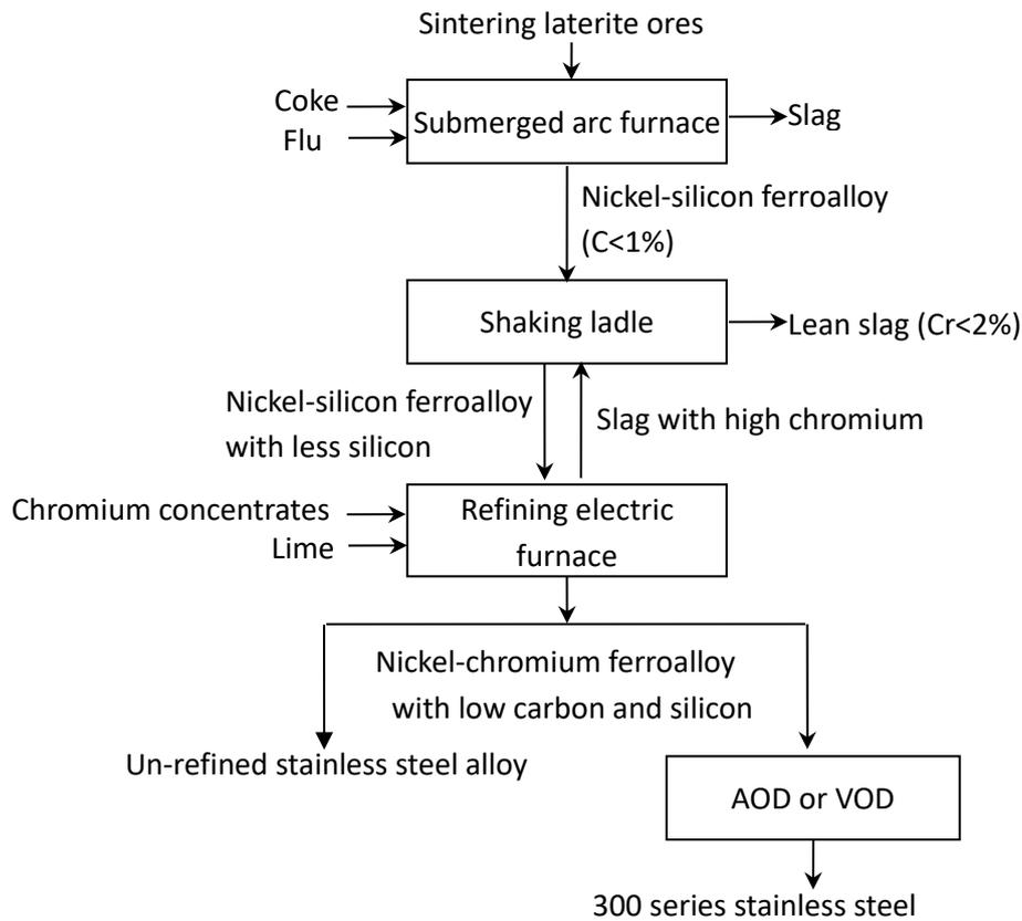
Figure 1. 300 series stainless steelmaking process with electric-silicothermic method.
