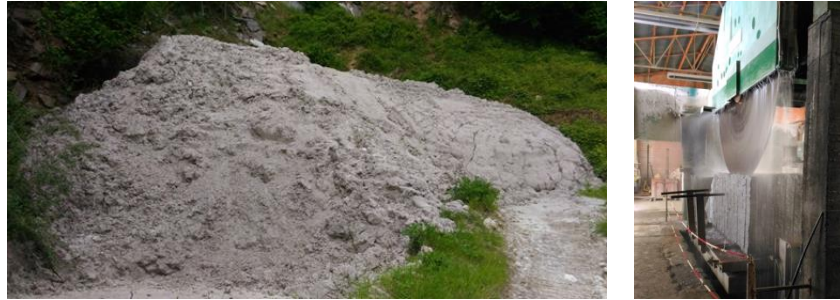
Figure 2: Company 1 (Perosa) – cutting methodology: diamond blade (on right) – open-air sludge disposal (on left)
