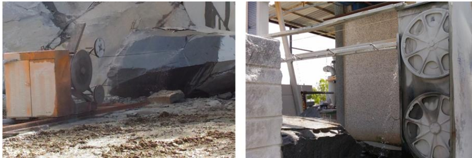
Figure 3: Company 2 (Diorite Traversella) – cutting technology for the extraction (on left) and for the processing (on right): diamond wire
