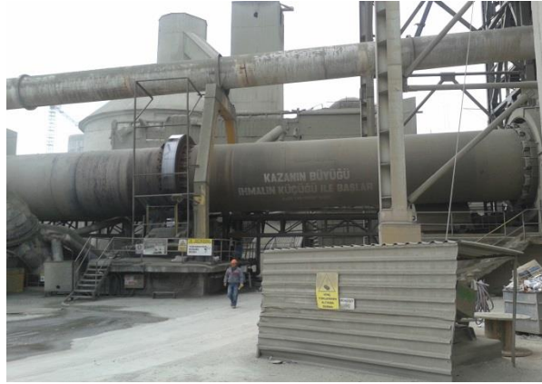
Fig.1. Clinker production in rotary kiln.
