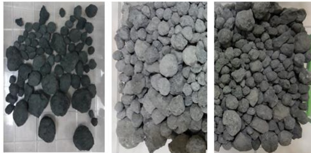
Fig.2. Clinker samples produced from 1 wt. %, 2 wt. % and 3 wt. % CSW containing raw meal, respectively.
