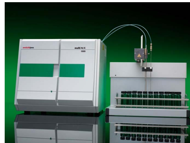
STOC and STN analyses performed by AnalitikJena Multi N/C Analyzer
