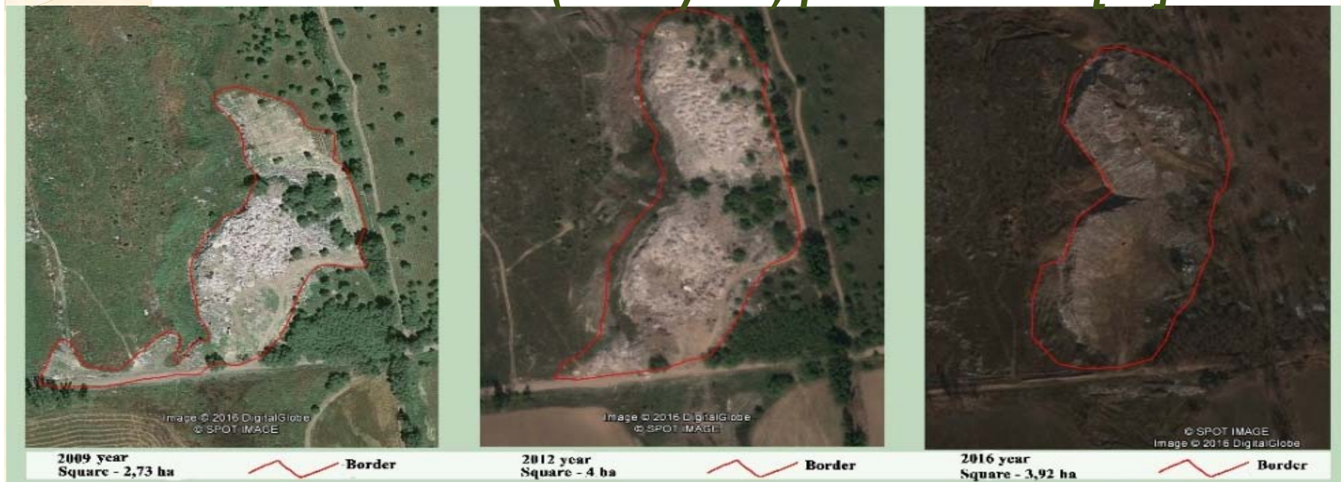
Figure 6 - Dynamics of changes in the boundaries of the dump near the settlement KIZ (Almalybak) for 2009-2016. [28]
