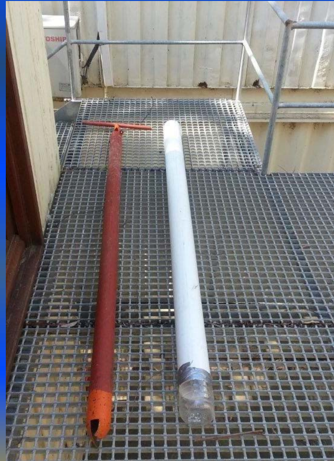
Figure 1: The hollow sampler that was used to collect the pit latrine faecal sludge on the first sampling expedition with the plastic cover sleeve next to it.
