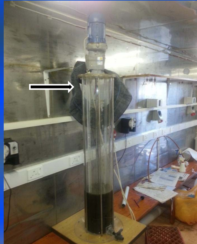
Figure II: The Perspex digester used for anaerobically digesting pit latrine faecal sludge. An inner tube of a car tyre (white arrow) was attached to the top of the digester collected biogas.
