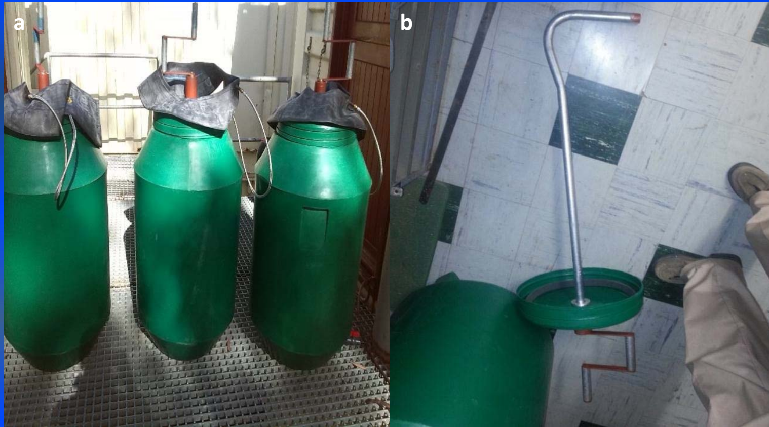
Figure III a: The second type of anaerobic digesters with the attached inner car tyre tube. Figure III b: The crank handle with the stirrer attached to the lid of the anaerobic digester. This was to permit stirring of the anaerobic digester contents.
