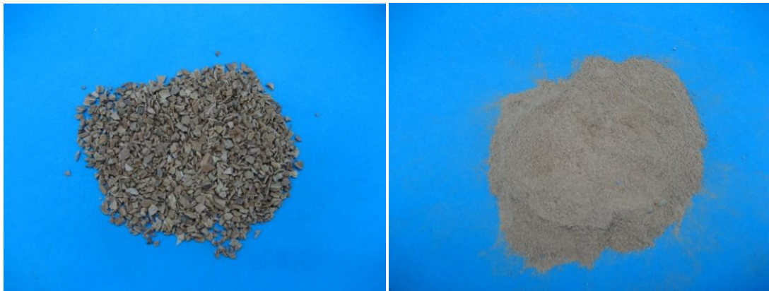
Figure 2. Milled Almond Shell: Size Particles less than 5 mm (left). Size Particles less than 1 mm (right)
