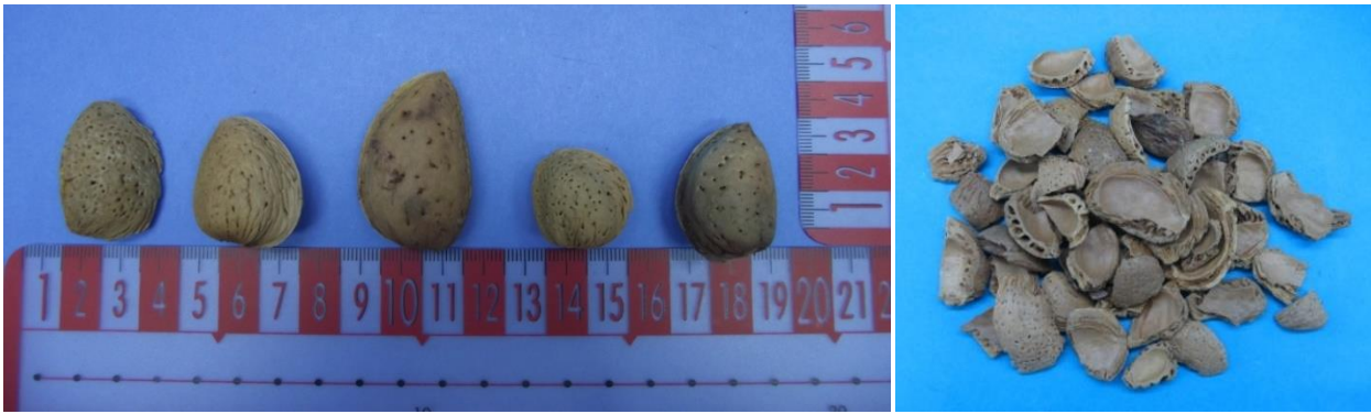
Figure 1. Almond shell varieties used: Comuna, DesmayoRojo, Largueta, Marcona and Guara (left). Mixed varieties, supplied in fragments (right)
