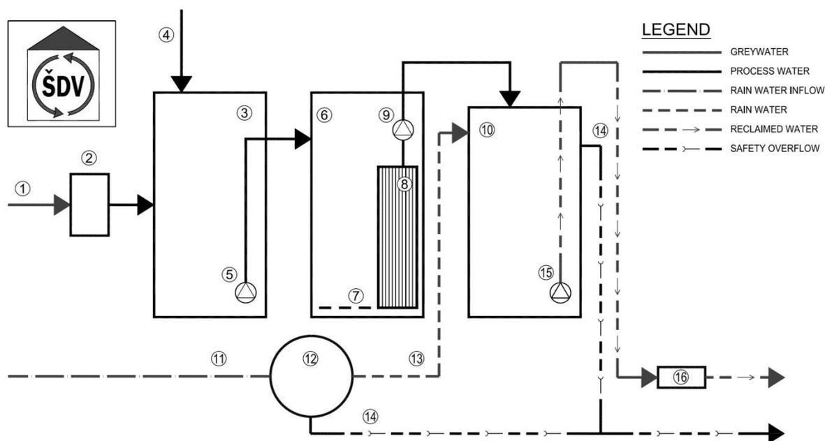
Fig. 1 Process diagram of an MBR treatment unit (legend: 1-greywater inflow, 2-mechanical pre-treatment, 3-expansion tank, 4-chemical dosing, 5-pump, displacement into biological unit, 6-biological unit, 7-activation, 8-MBR unit, 9-pump, displacement into storage tank, 10-storage tank, 11-rainwater inflow, 12-rainwater storage tank, 13-rain water draw-off into storage tank, 14-safety overflow into sewer system, 15-automatic booster station, 16-hygienic safety unit)
