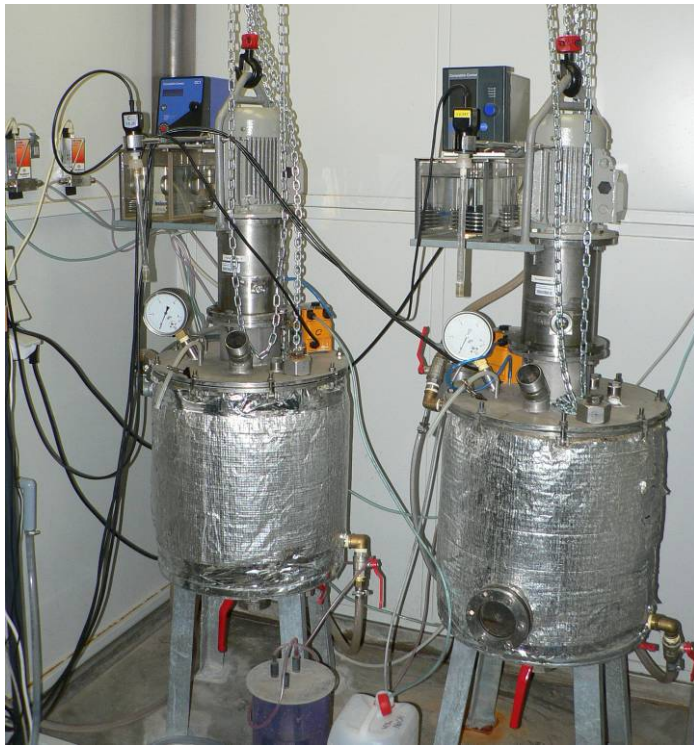
Fig. 2 Photo of the anaerobic laboratory digesters
