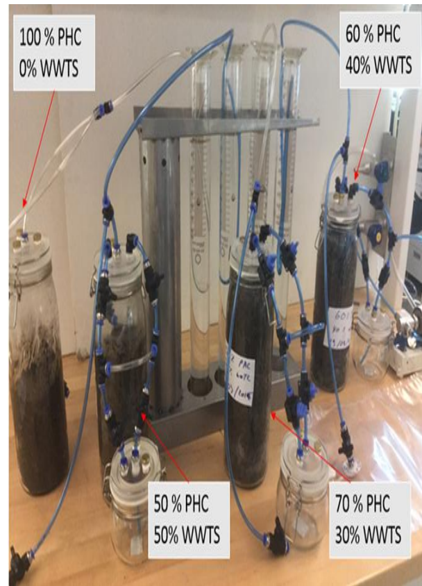
Fig. 3: Experimental reactors setup
