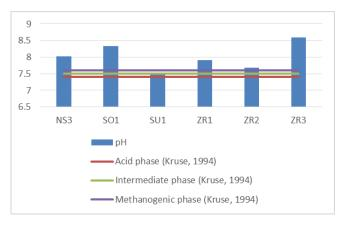
$\textbf{Fig. 2} \ \ \textbf{Estimation of degradation phase in relation to} \\ \ \ \textbf{literature values for pH}.$
