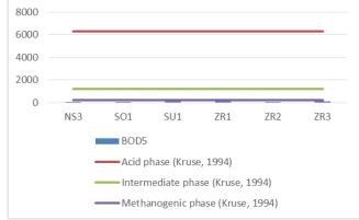
**Fig. 3** Estimation of degradation phase in relation to literature values for BOD5.
