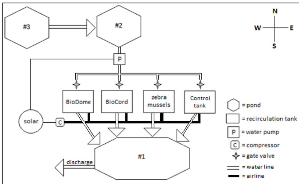
**Fig 1.** Experimental setup for testing of biofilm technologies at Storrings Septic, weeks 1-14. During weeks 15-20 of summer testing, the zebra mussel tank was decommissioned, leaving the three remaining tanks for use in our research. Image not to scale.
