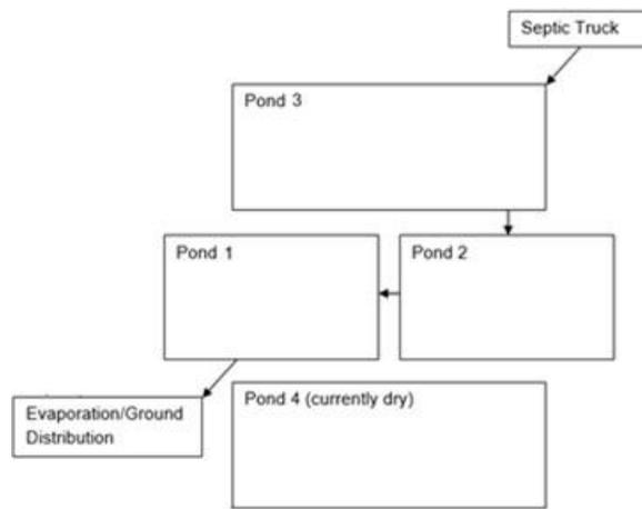
**Fig 12.** Diagram of the typical process flow currently in use. Arrows indicate direction of the inflow/outflow of wastewater.
