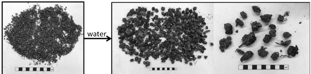
Fig. 10 Agglomeration of fine grain due to a water content of 50 wt.-%
