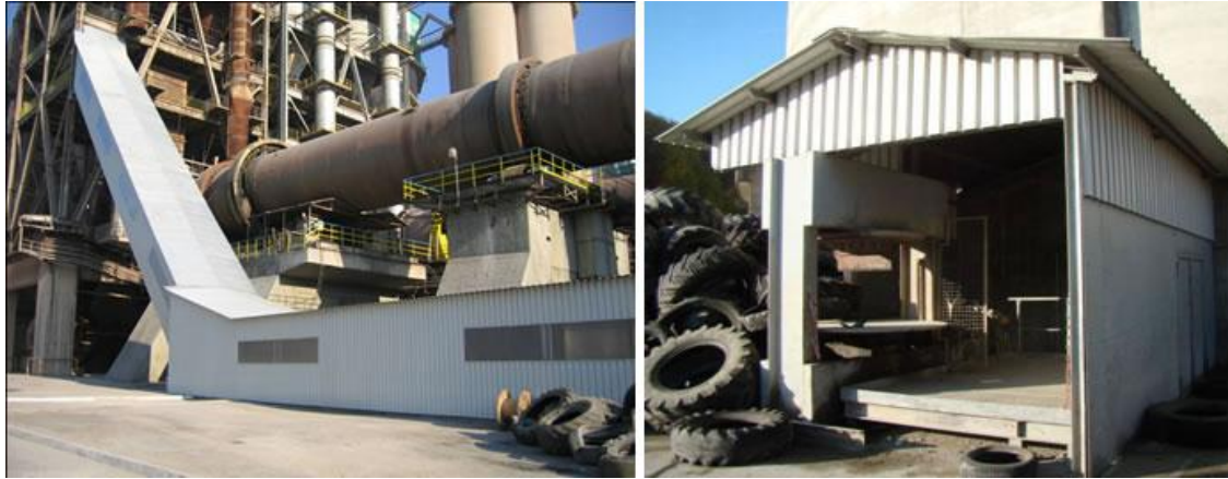
Figure 3 System for processing of large tires to be used as alternative fuels in cement kilns
