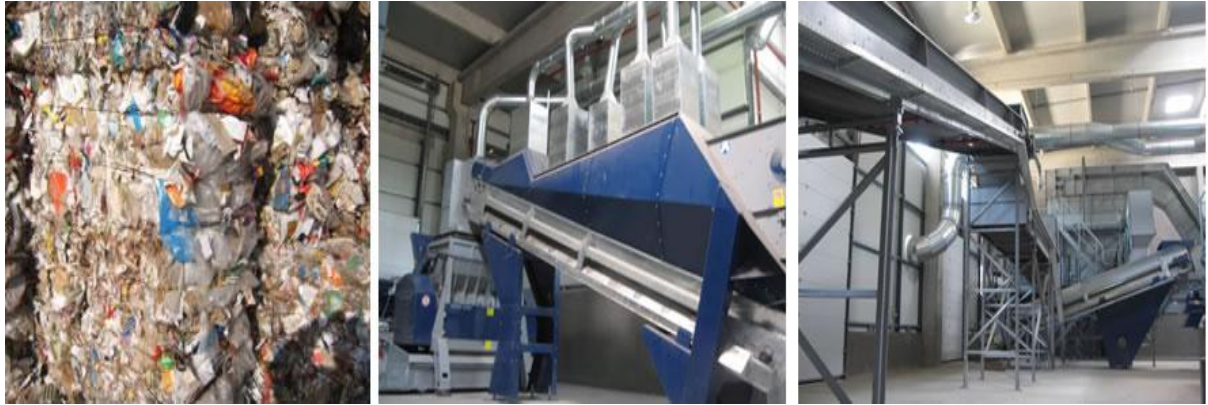
Figure 4 System for processing of plastics, paper and cardboard to be used as alternative fuels
