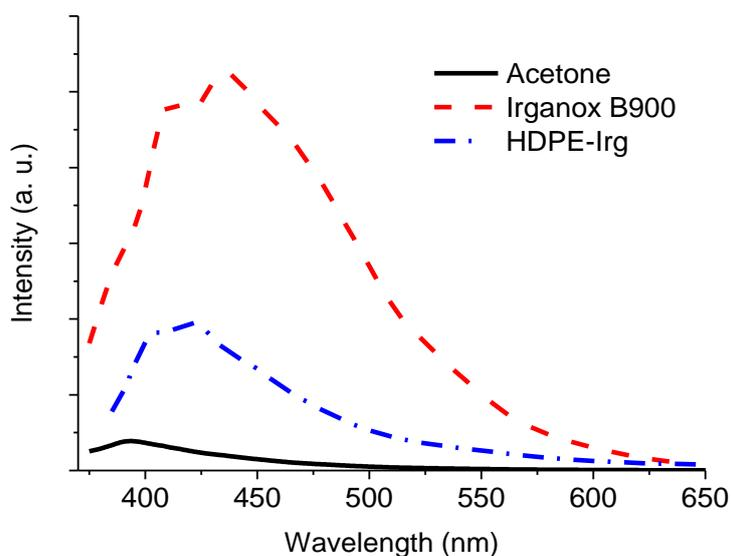
**Fig. 3** Fluorescence emission spectra ( $\lambda_{\text{ex}} = 350 \text{ nm}$ ) corresponding to Irganox<sup>®</sup> B 900 (solution in acetone) and the HDPE used in this work (0.2 wt % of Irganox<sup>®</sup> B 900)
