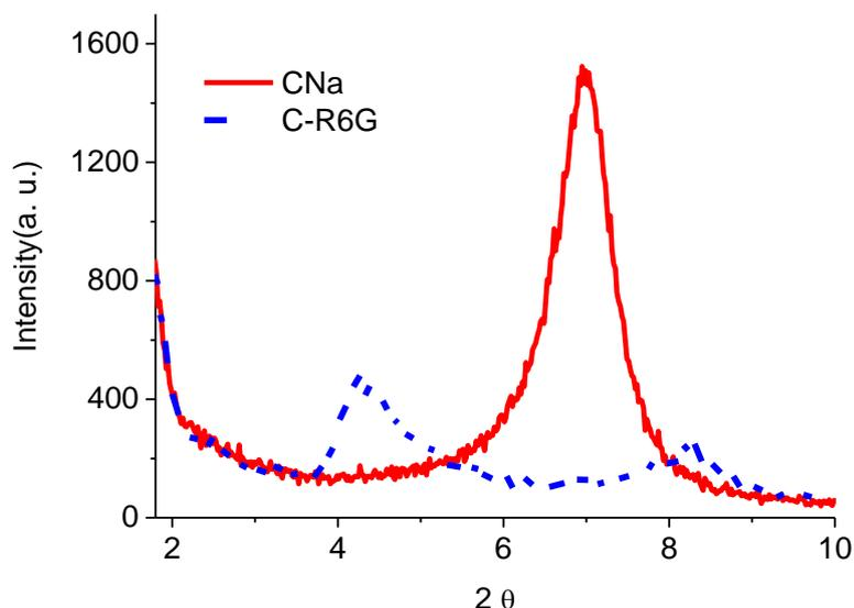
**Fig. 4** XRD traces corresponding to unmodified clay (CNa) and CNa modified with R6G
