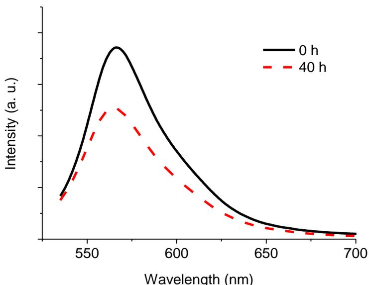
**Fig. 8** Fluorescence emission spectra ( $\lambda_{\text{ex}} = 510 \text{ nm}$ ) corresponding to HDPE labeled with R6G before (solid line) and after (dashed line) 40 h of thermal treatment at  $80 \text{ }^\circ\text{C}$
