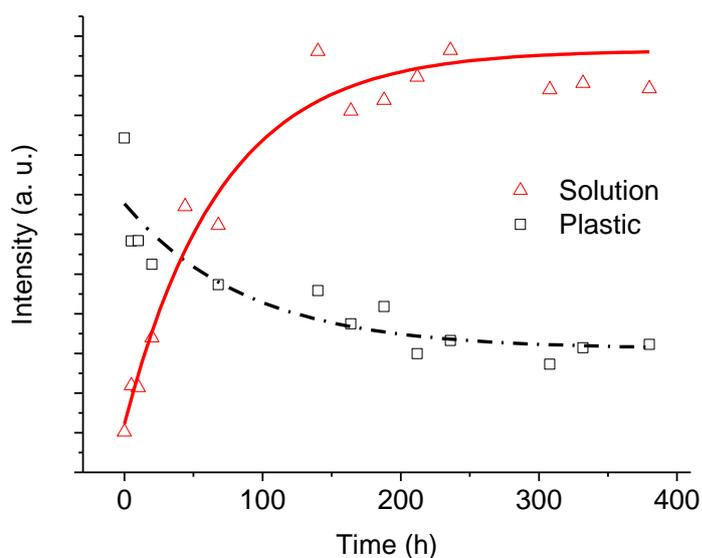
**Fig. 10** Time evolution of the emission intensity ( $\lambda_{\text{ex}} = 510 \text{ nm}$ ) of HDPE marked with R6G and its immersion medium during the hydrothermal degradation
