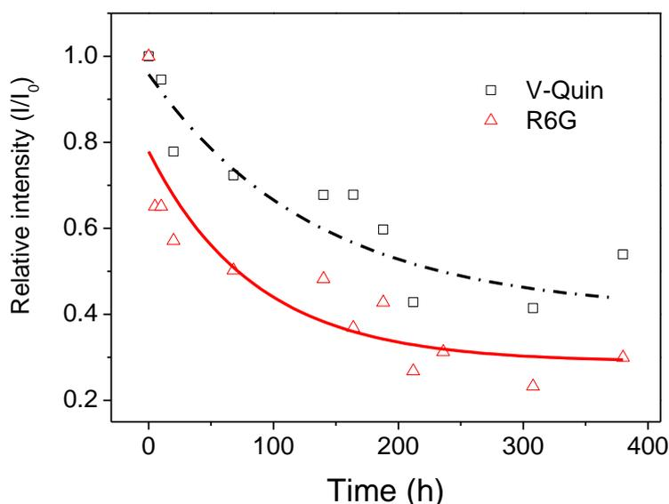
**Fig. 13** Retention of the fluorescence emission of HDPE marked with R6G and V-Quin during the hydrothermal degradation
