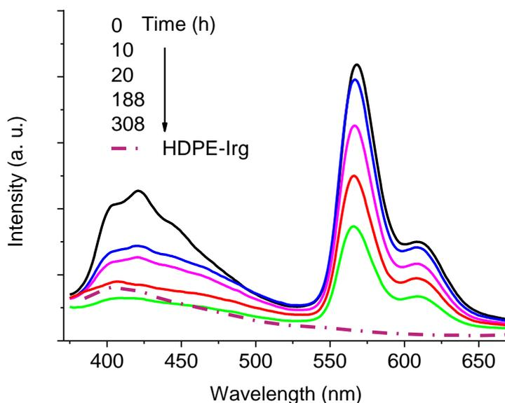
**Fig. 12** Evolution of the fluorescence emission of HDPE marked with V-Quin ( $\lambda_{\text{ex}} = 350$  nm) during the hydrothermal degradation
