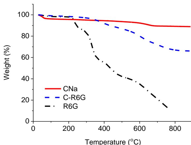
**Fig. 5** Thermogravimetric traces corresponding to unmodified clay (CNa), R6G and CNa modified with R6G
