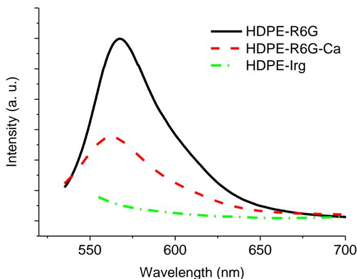
**Fig. 6** Fluorescence emission spectra ( $\lambda_{\text{ex}} = 510 \text{ nm}$ ) corresponding to HDPE labeled with R6G (10 ppm, solid line), HDPE labeled with R6G and containing 10 % by weight of  $\text{CaCO}_3$  (dashed line) and to unlabeled HDPE (dash dot)
