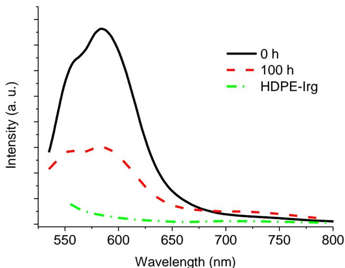
**Fig. 7** Fluorescence emission spectra ( $\lambda_{\text{ex}} = 510 \text{ nm}$ ) corresponding to HDPE (with 10 wt% of  $\text{CaCO}_3$ ) labeled with R6G-modified clay, measured before (solid line) and after (dashed line) 100 h of photochemical degradation
