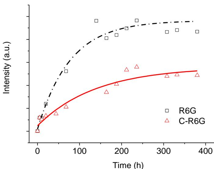
**Fig. 11** Time evolution of the emission intensity of the immersion media ( $\lambda_{\text{ex}} = 510 \text{ nm}$ ) during the hydrothermal degradation of HDPE marked with R6G and R6G-modified clay
