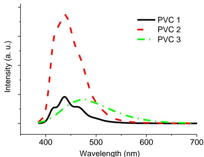
**Fig. 1** Fluorescence emission spectra ( $\lambda_{\text{ex}} = 350 \text{ nm}$ ) corresponding to three commercial samples of PVC
