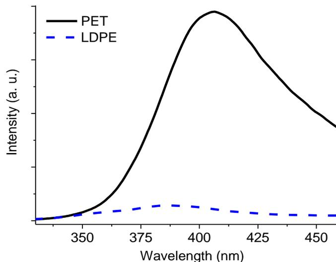
**Fig. 2** Fluorescence emission spectra ( $\lambda_{\text{ex}} = 290 \text{ nm}$ ) corresponding to commercial samples of PET and LDPE
