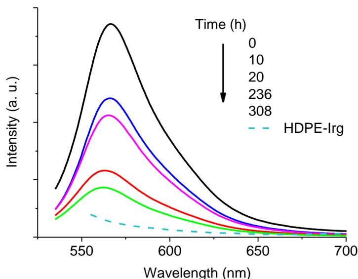
**Fig. 9** Evolution of the fluorescence emission of HDPE-R6G ( $\lambda_{\text{ex}} = 510 \text{ nm}$ ) during the hydrothermal degradation
