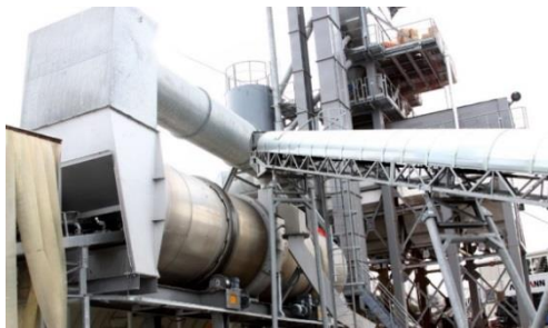
Figure 7. Drying oven and installation of sieves and mixer
