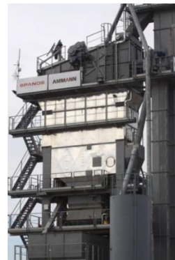
Figure 7. Drying oven and installation of sieves and mixer
