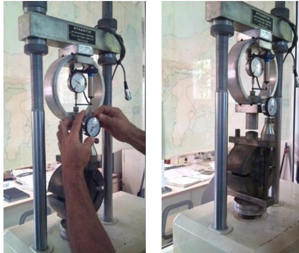
Figure 11. Marshall test (stability and deformation of bituminous mixture)
