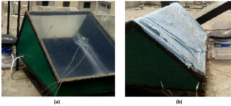
Fig 2. (a) Still when secondary cover is bare (b) Still when secondary cover is covered with wet cotton cloth
