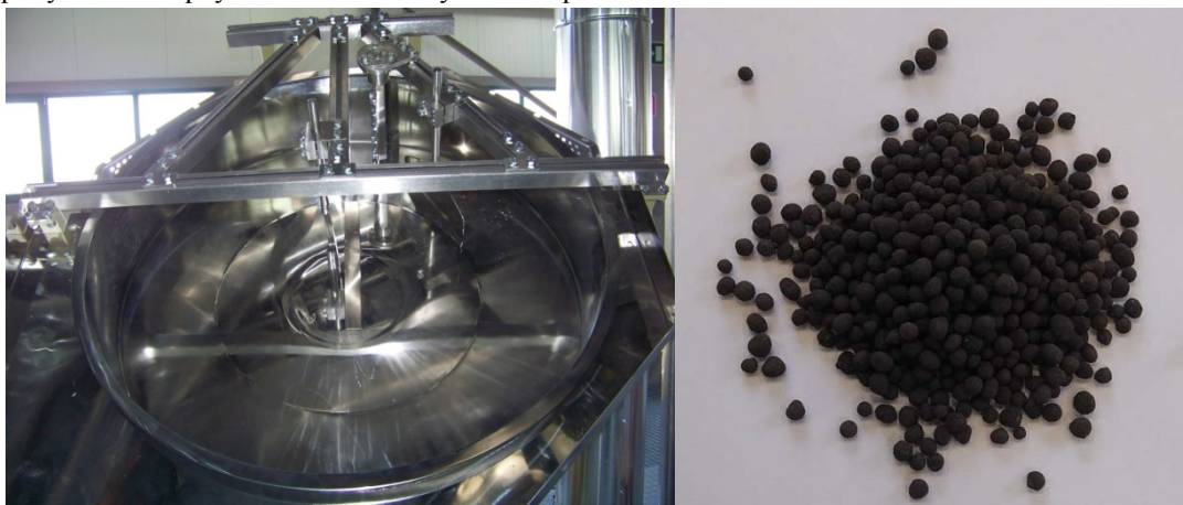
Drawing 1. On the left: granulation plate used in semi-technical tests. On the right: granulate obtained in tests
