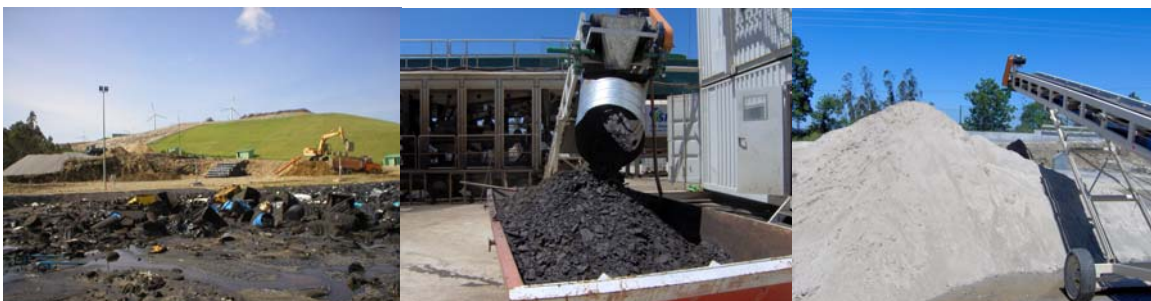
Picture series 1. Prestige shipwreck waste (left), high caloric filter cake (middle), recovered sand (right)
