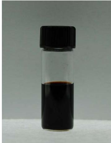
**Fig. 11:** Final concentrate of the extracted phenols from olive leaves, after vacuum evaporation of the resin ethanolic effluent.
