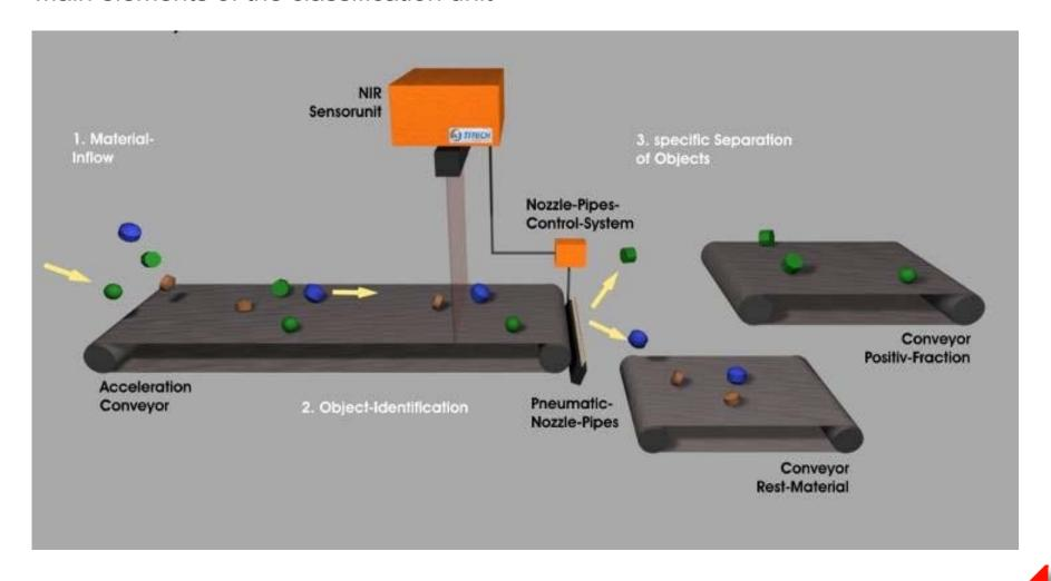
Material identification through NIR (Near InfraRed) Wavelength spectrum of NIR
