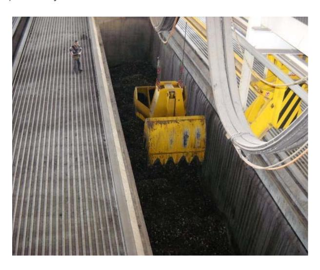
Bioreactors are special constructions equipped with perforated concrete plates. Through those plates a controlled air stream is guided to the waste matrix so that the material is evenly aerated. All critical parameters of the process are constantly monitored and recorded. By this way the operator can adjust all crucial parameters (matrix temperature, matrix moisture, oxygen concentration) and ensure the successful and on-time completion of the process.
