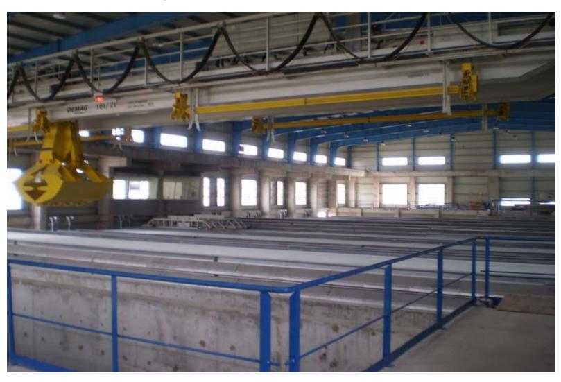
The separated fine fraction of the waste, very rich in organic matter, is collected and submitted to intensive aerobic composting process in order to be stabilized. After the completion of this process the stabilized fraction is stored in piles and is mechanically aerated (by means of a compost turner) until its maturation.
