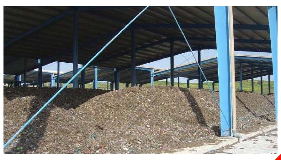
After completion of the intensive composting, the fine fraction of the waste is put in piles in a dedicated covered area. The material stays for a period of five to six weeks, periodically mechanically mixed, until its maturation is completed. For the mixing of the piles a special vehicle (compost turner) is used.
