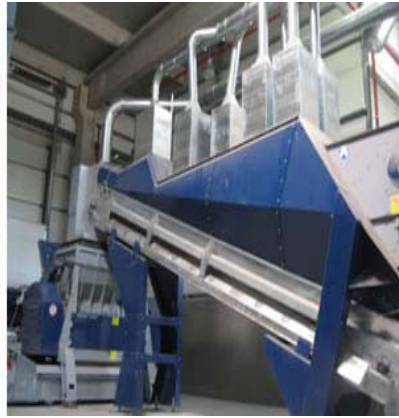
System for processing of plastics, paper and cardboard to be used as alternative fuels
